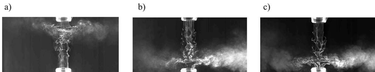
Figure 4. Smoke-wire photos at L = 4D , a = 1 \pm 1\% (a and b) and 0.97 (c).
